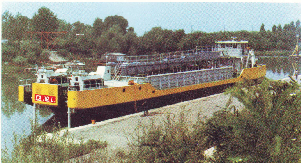
DVM/R range propulsion units on a mobile dredger.
